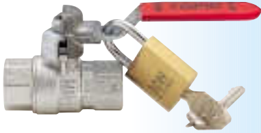
Full bore ball valve, female/female, with steel handle, lockable in closed and open position by means of a padlock, nickel-plated. Art. S.0200 without padlock Art. S.1200 with padlock
